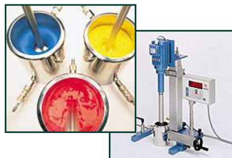
Dispersion process, e.g. dissolver
